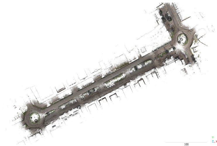
Fig. 5. Point cloud from CHCNAV RS10 of Via Primo Maggio – orthogonal view in CloudCompare.
