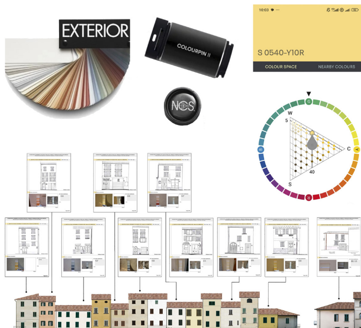
Fig. 6. Natural Color System (NCS) Palette and Colorpin; the example of façade colour survey and building recording for Terranuova Bracciolini historic centre (2014) coordinated by the author.
